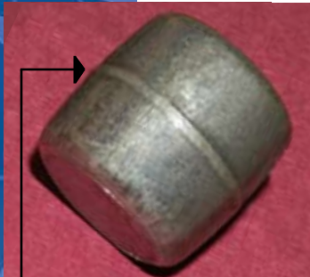
Traditional cold formed part with a flash band imperfection.
